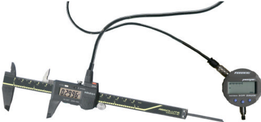
Visor with DataGet BCD cartridge connected to Mitutoyo 6" caliper, and Mahr Federal \mu Max1µm indicator
